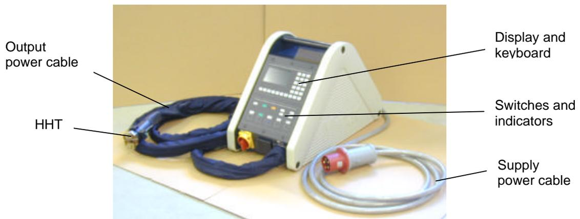
Figure 1. MINAC Standard 25/40 Induction Heater.
