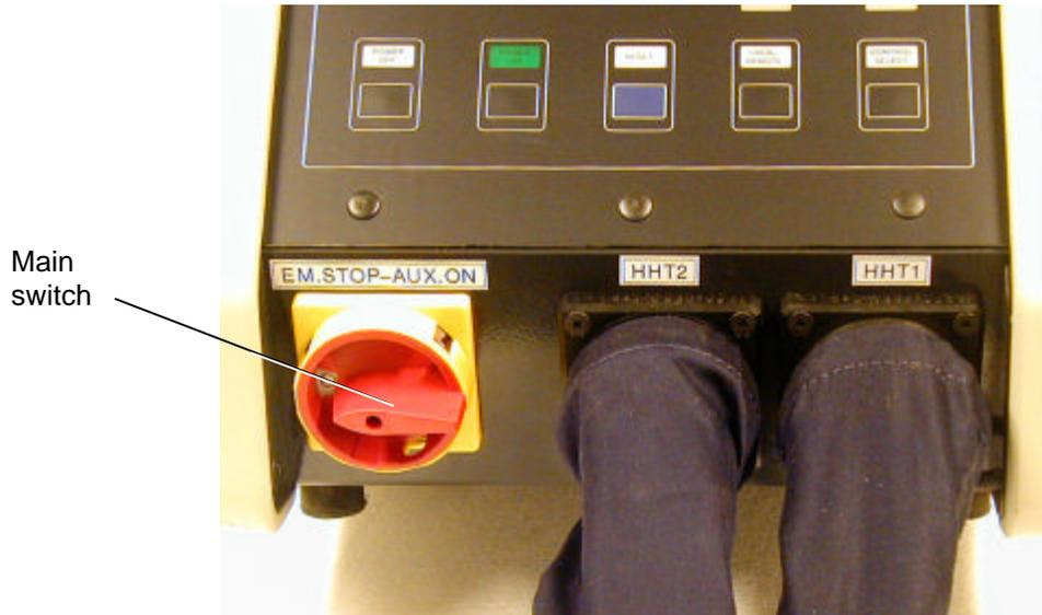
Figure 11. MINAC 25/40 and 50/80 cabinet front, main switch
