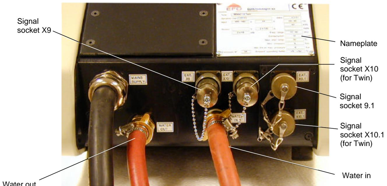
Figure 8. Supply input/output panel on rear of cabinet.
