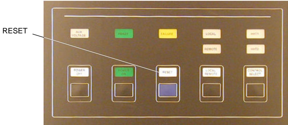
Figure 13. Switches and Indicators panel, RESET button
