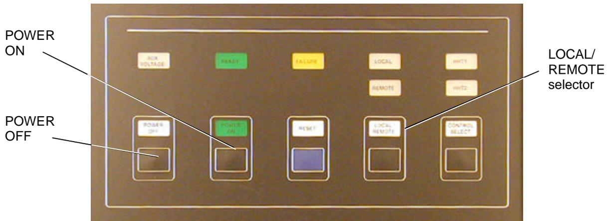
Figure 12. Switches and Indicators panel, POWER ON/OFF buttons
