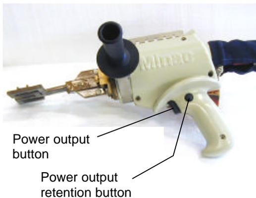
Figure 9. HHT 240S, power output and retention buttons
